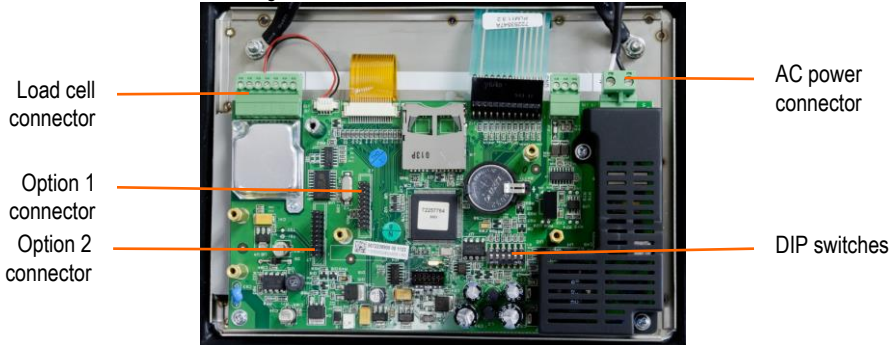
Figure 1-3: T72XW Main Board Connections, AC Model
