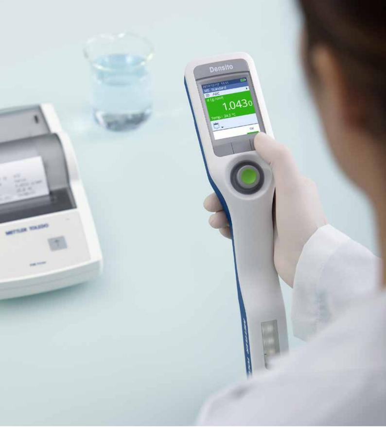
The density of a liquid can be used as a unique identifier in quality control. Ensure the highest quality by setting up a range of acceptable limits for your samples: results that fall within this range are color-coded, enabling instant identification of acceptable samples.
