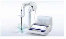
Keep your sensor up to speed Clean the sensor with DI water after each measurement, store in-between measurements in InLab Storage Solution and periodically re-condition it in 0.1M HCI to ensure fast response.
