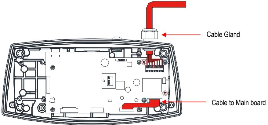
6. Connect the load cell cable to the terminal block (J1).
