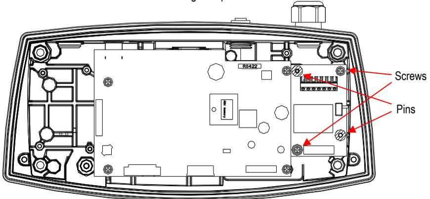
5. Install the cable gland, and pass the load cell cable through it. Connect the cable between the A/D board and Main board.
