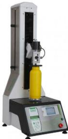
Topload , for automated crush tests on bottles
