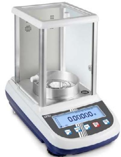
**KERN ALJ 200-5DA** with optional ioniser
