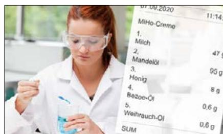
Clear printout with date and time. In addition, the components of the mixture are numbered automatically and printed out with the name & weight
