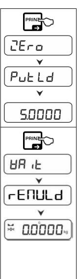
⇒ Acknowledge selection by →-button. < ☐E □ →, < ☐E L☐ >, < ☐E L☐ > followed by the weight value of the adjustment weight to be placed will be displayed.
