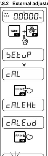
⇒ Press and hold the TARE and ON/OFF buttons simultaneously to enter the setup menu.
