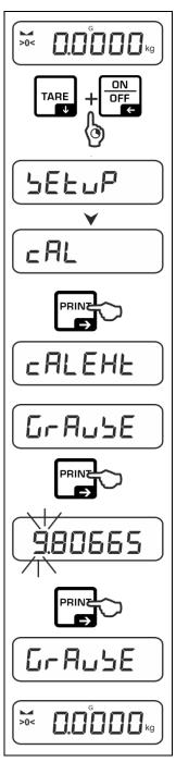
⇒ Press and hold the TARE and ON/OFF buttons simultaneously to enter the setup menu.
