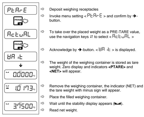
The entered tare weight remains invalid until a new tare weight is input. To delete press the TARE key or confirm the menu setting <□ LEH□> using the → button.
