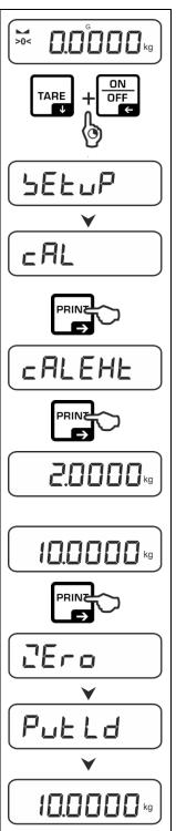
⇒ Press and hold the TARE and ON/OFF buttons simultaneously to enter the setup menu.
