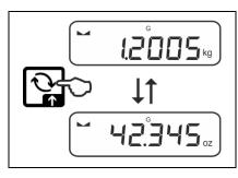
Using 5 button, it is possible to switch over between the enabled unit 1 and unit 2.
